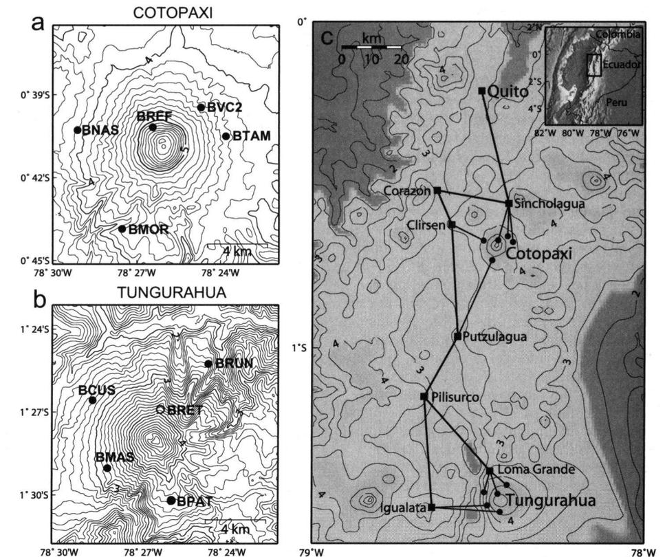
Fig. 2. Locations of broadband seismic and infrasonic stations at (a) Cotopaxi and (b) Tungurahua volcanoes. The open circle in the Tungurahua map shows the location of the station yet to be installed. (c) Digital radio telemetry routes from the observation stations at Cotopaxi and Tungurahua (circles) to the central office in Quito via repeaters (squares). The rectangle in the inset shows the area featured in Figure 2c. Original color image appears at the back of this volume.
